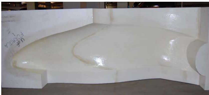
One half of the body mold during preparation process. Mold kindly provided by Art Attack.
